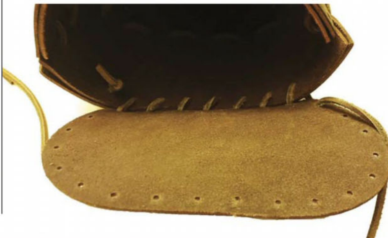
Start your lacing a few holes in from where the two pieces of the quiver body come together. This will make it easier to run the lace through the holes when you get closer to the end.
