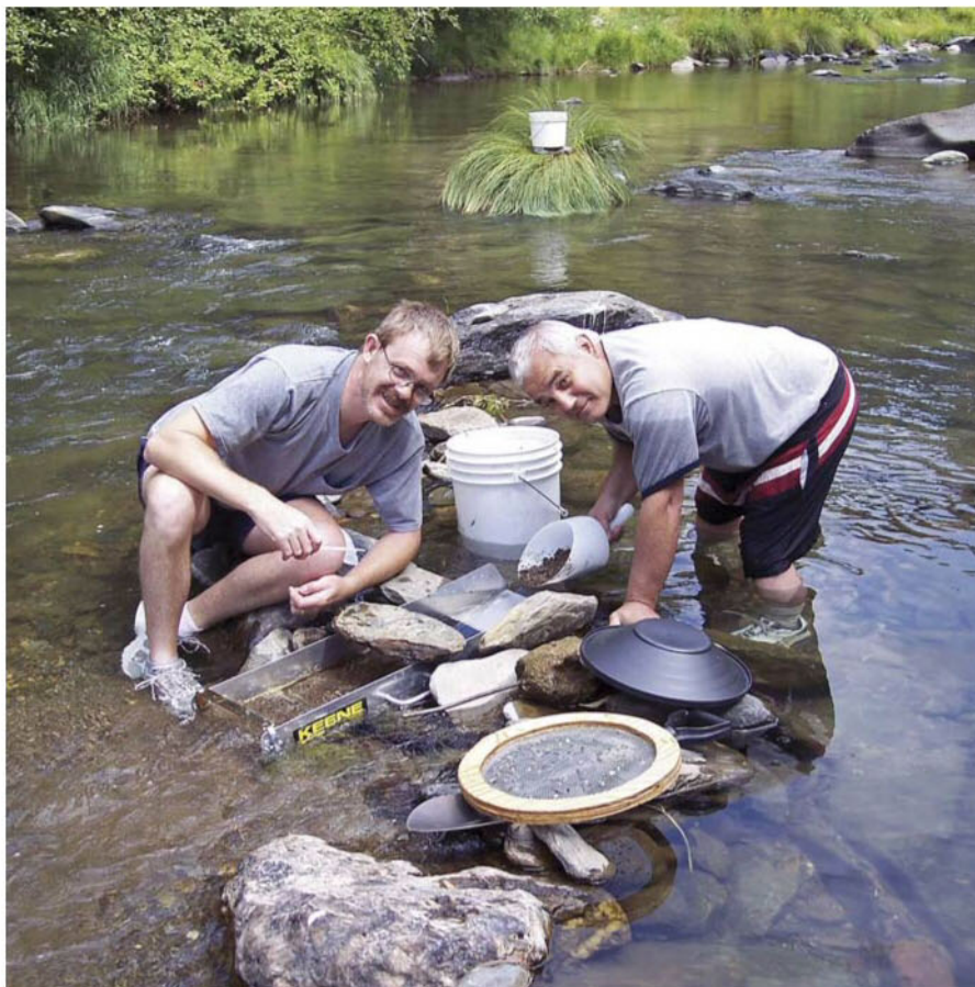
(above) Indiana prospector Tom Smith (left) and friend Chip Hinchman scoop material into a sluice box. Pictured in the foreground is one of Smith's homemade classifiers. (below) Pictured in this pan: approximately 1½ grams gold. It takes 31.1034768 grams to make 1 troy ounce of gold.
