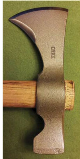
The CRKT Woods Chogan is a drop-forged tomahawk shaped with a blunt hammer, which makes the steel very dense and strong. It is the heaviest of the hawks discussed in this article and has the longest cutting edge—resulting in a very effective tool for use in camp, at home or on the hunt.
